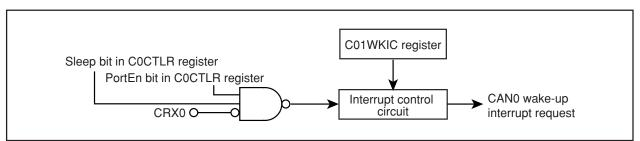
Figure 9.15 CAN0 Wake-up Interrupt Block Diagram
